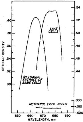
Figure 5. Absorption spectrum of *Chlorella* and pigments from *Chlorella*, (measuring band width 1 m $\mu$ , after Cederstrand).
